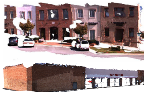
Figure 6. Reconstructed buildings using stability-based fusion
