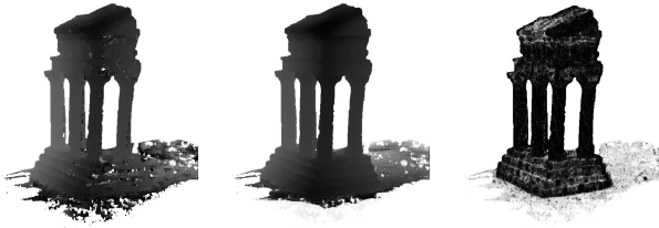
Figure 3. A stereo depth map for a dataset from [19], the fused depth map using stability-based fusion and the final confidence map (black corresponds to maximum confidence).
