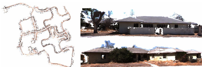
Figure 1. Aerial View and Detailed Views of reconstructed models from a 170,000 frame video
