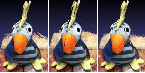
Figure 6: Reconstruction results for our three different settings. From left to right: ours , ours comp , ours fast . Note how the complete version is able to close the holes around the eye but suffers from boundary artifacts along the crest. On the other hand, the fast version, similar to the original, presents bigger holes around the eye and on the right side of the mantle.
