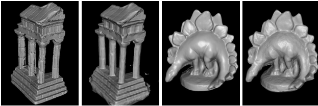
Figure 8: Ground truth surfaces and reconstructions for Temple Full and Dino Full of the Middlebury multiview stereo evaluation dataset [34].
