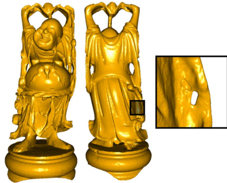
Figure 7: Stanford happy buddha . 380K vertices, 738K triangles. Setting the tolerance parameter \sigma too high might create unwanted holes (inside the square).
