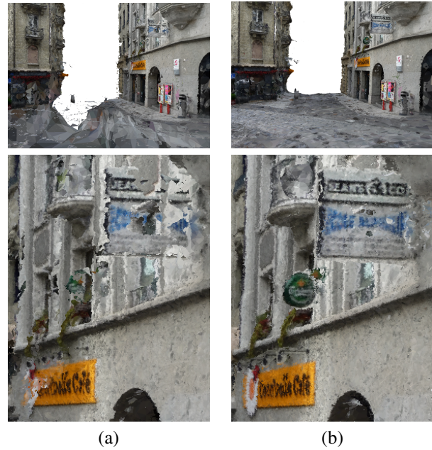
Figure 8. Results for the 'strecha' data set. (a) reconstruction using our implementation of the base-line approach, (b) reconstruction using our approach. Weakly-supported surfaces are better reconstructed using our approach than by base-line approach.
